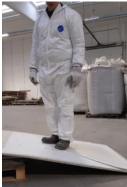
Figure 8: No deflection with a 100 kg man (Gees Recycling, 2019)
