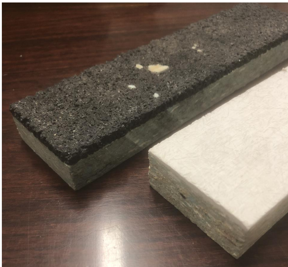
Figure 5: Left co-moulded Recycled Fibre Material (RFM) & recycled rubber, right co-moulded RFM & SMC (Gees Recycling, 2020)
