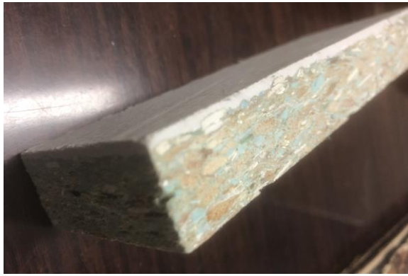
Figure 6: Layer of SMC (white) co-moulded on RFM (Gees Recycling, 2019)
